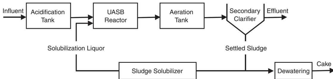
**Fig. 9 – Schematic of a wastewater treatment system with solubilization producing less sludge (modified from Saiki et al., 1999).**
