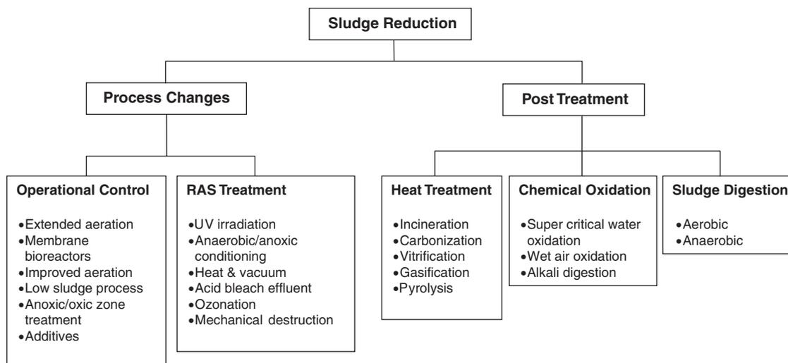
Fig. 1 – Outline of sludge reduction technologies.
