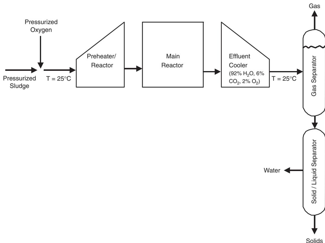
Fig. 8 – Schematic of a SCWO system (modified from Modell et al., 1992).
