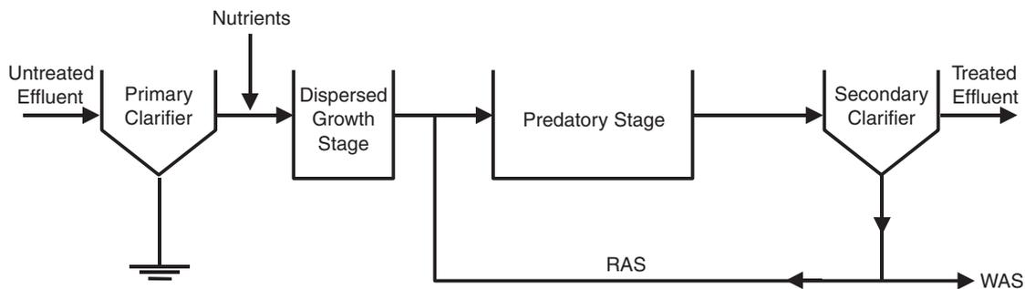
Fig. 4 – Schematic of the two-stage low sludge process.
