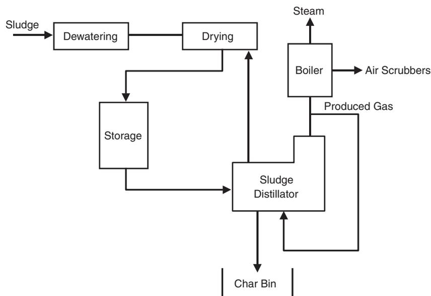
Fig. 6 – Schematic of the sludge carbonization process (modified from Nichols, 1992).
