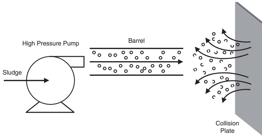
Fig. 10 – Schematic of high pressure impact for sludge pretreatment (modified from Nah et al., 2000).
