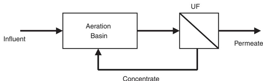
**Fig. 2 – Schematic of a membrane bioreactor.**
