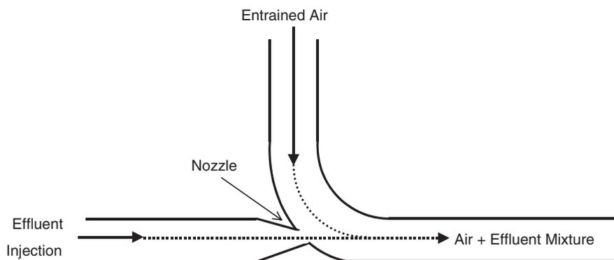
Fig. 3 – Conceptual diagram of a Venturi injector (modified from Young and Barlow, 1998).
