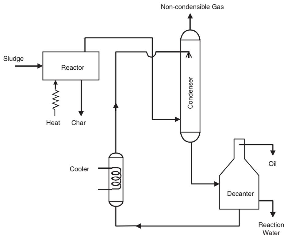
**Fig. 7 – Schematic of a sludge to oil converter (modified from [Campbell, 1989](#)).**
