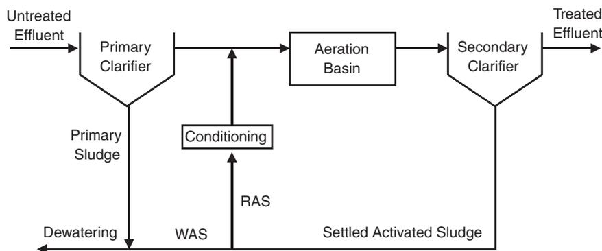
Fig. 5 – Schematic of recycled sludge conditioning.
